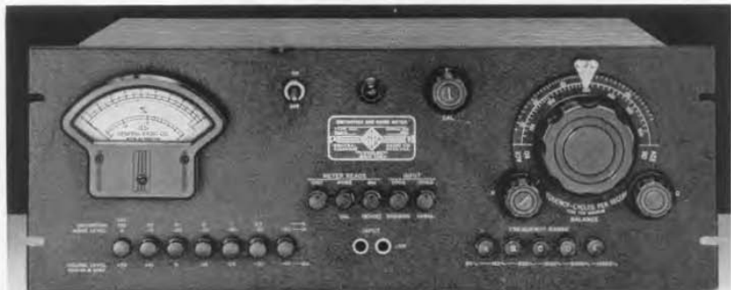
Figure 1. Panel view of the Type 1932-A Distortion and Noise Meter.
